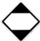
Limited Quantity Ground
